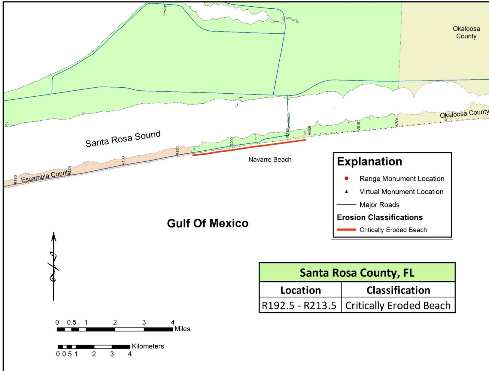
Figure 16. Critically eroded shoreline within Santa Rosa County.
