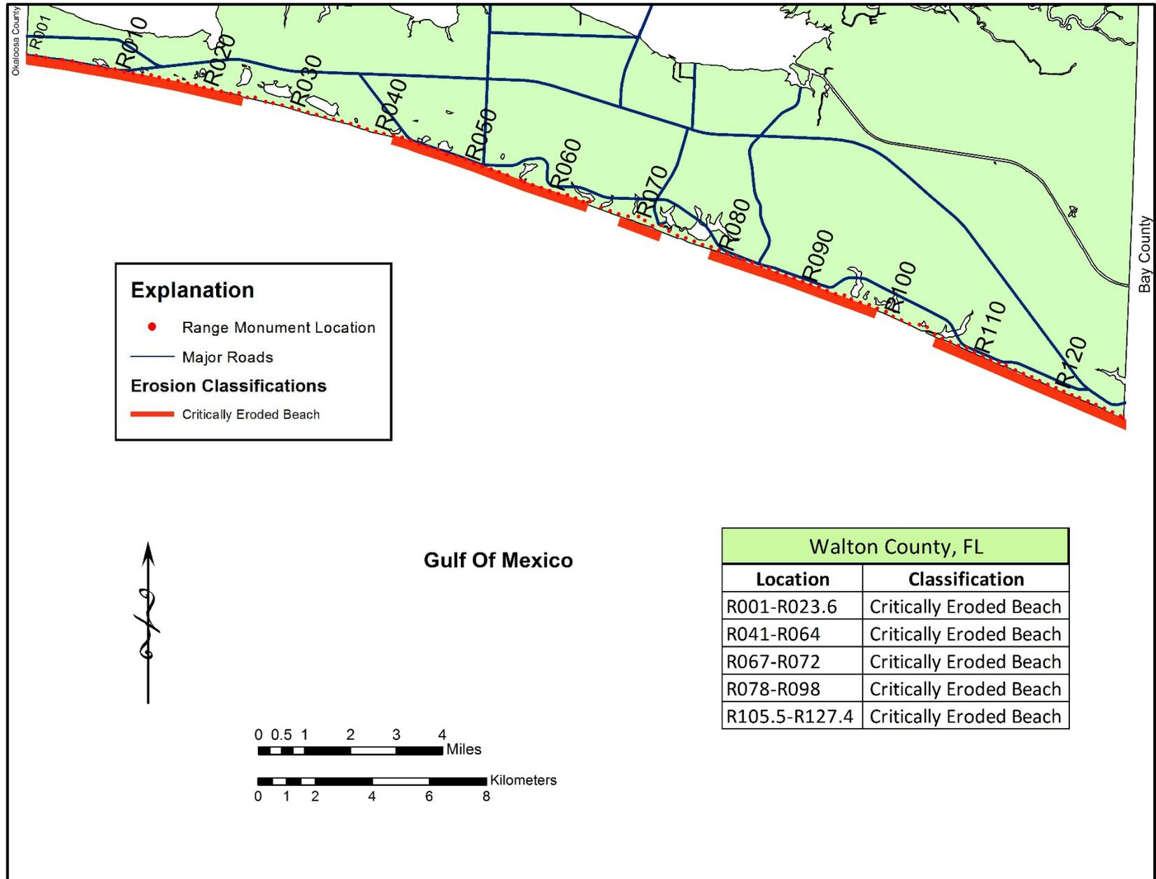
Figure 18. Critically eroded shoreline within Walton County.
