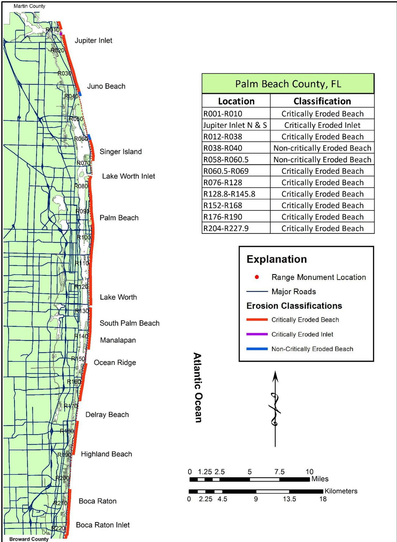
Figure 11. Critically eroded shoreline within Palm Beach County.
